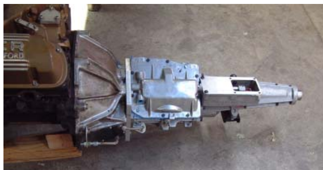
Fig 5 Here's the assembly ready for installation. Note that the Shifter mechanism has been removed, but the cover plate remains in place. It won't go into place with the shifter installed.
