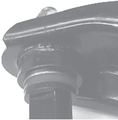
Figure 10. A closeup of the skip weld on the lower bushing shell. This is an important safety modification. Stock spin wells have been known to fail.
