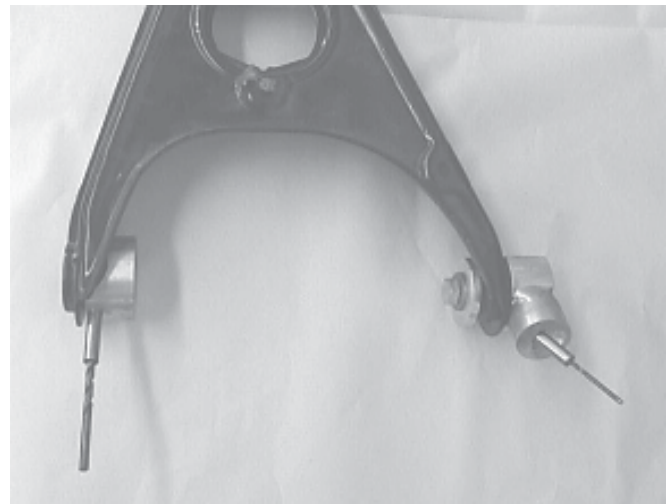
Figure 5. This view shows the straight and angled fixtures for the Lower A-Arms. If you choose to drill your Arms for fittings, you would install the rear bushing first so that you could still re-install the drill guide and drill through the shell and urethane media before the fulcrum pin is installed.
