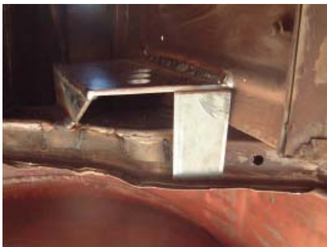
Figure 12. The last piece to place is the clip from the bottom the the frame flange. This piece adds the last piece of rigidity that make this kit stiff enough to stand up to substantial abuse or simply restore the OEM function with a better chance of survival.
