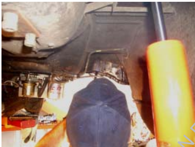
Figure 3. It's a little hard to see because of the head, but we're applying heat with a propane torch to soften and loosen the accumulated road dirt and undercoating. You're also working adjacent to the fuel lines and pump, so your going to want to be sure that there is no fuel seepage and vapors in this area before you light up the torch.
