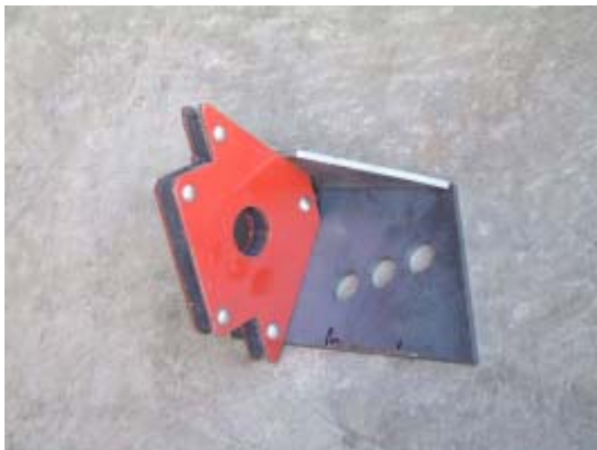
Figure 8. The magnetic clamp makes a nice right angle for the weld setup. The two plates are the same length making alignment pretty easy.
