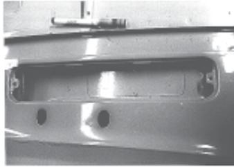
outside of the vent shell. The side dimension on the right side was 1.45", and on the left it was 1.70". The front to rear measurements were taken from the cowl wall below the recessed lip, to the rear outside of the shells. They are .375" to .437" on both sides. This dimension is
