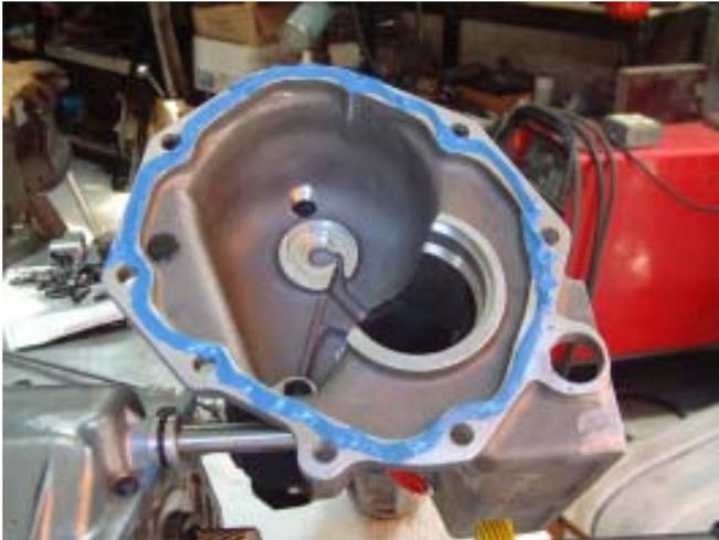
**Fig. 24** Here's the typical application of RTV on the sealing face of the tailhousing. You don't need it around the top ring, the O-ring on the cover does the sealing in that location. A dab of grease on the O-ring makes assembly smooth.
