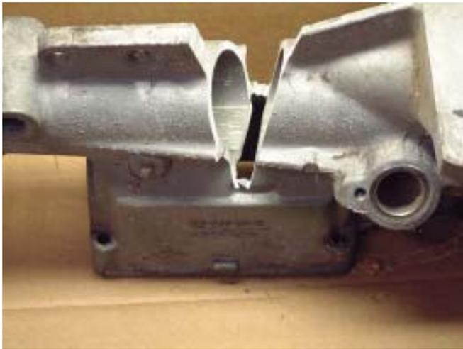
**Fig. 16** Here's another alternative for gaining access to the Shift Gate. By sawing a vee out of the housing, you can open a slot to place a drift to drive it out.
