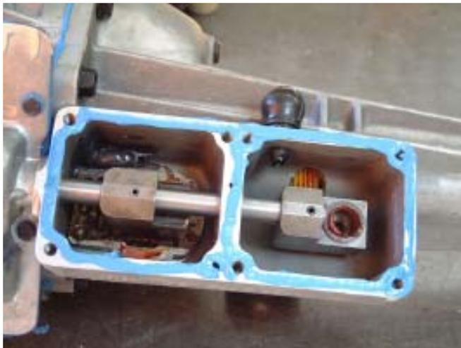
**Fig. 28** Here we have the shift box assembly complete. The vent bulb is installed and the bushing for the shift lever is greased and inserted in the rear shift block. RTV has been placed to seal this area.
