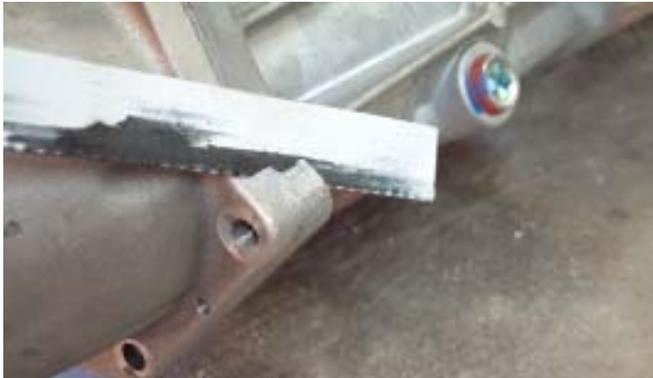
**Fig. 11** Start here at a slight angle to the rear but almost vertical.
