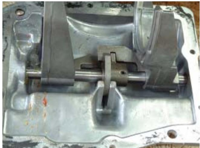
**Fig. 7** This is the working part of the Top Plate with the forks rolled to the side. You can see the 3/16 roll pin that keeps all these pieces assembled and in position. You may want to take notes and/or a digital shot of this mechanism as it will go together in different ways and only one is correct.
