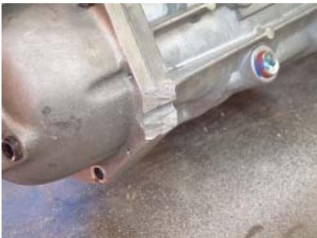
**Fig. 13** Here's our completed cut before grinding
