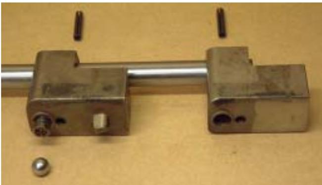
**Fig. 25** Here are the two Shift Blocks and related mechanisms supplied with the Kit. Note that the one on the right has been modified by sanding the peg off the bottom. They are displayed on the shift shaft in the correct positions. The Block with the peg goes in the forward box above the Shift Gate. The Block without the peg goes in the rear box and accepts the shift linkage.
