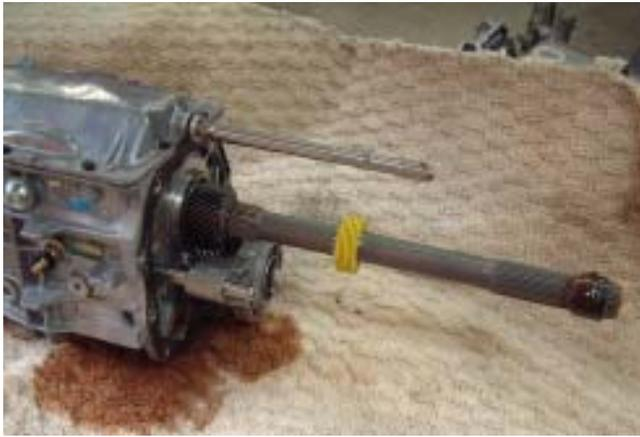
**Fig. 4** Here's the transmission with the tailhousing removed. Note the protruding shift shaft and the oil stain from disassembly. Save the rubber seal on the splines, it will seal on the input yoke of the longer driveshaft supplied in the kit.
