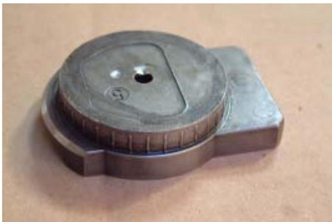
**Fig. 17** This is what the bottom of the shift gate looks like after it's pressed out. The tangs are all around the perimeter of the portion that is pressed into the housing. Breaking the leading edge with a sander will allow a little easier fir into the housing recess. Make very sure that this piece presses in straight, otherwise the tailhousing can be damaged or broken.
