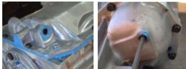
**Fig. 30** The screw threads on the 5/8-18 set screw are coated with RTV and this screw is used to close the hole in the top cover. The threads of the 3/8 pipe plugs are similarly coated and used to seal the drain and fill holes in the tailhousing.
