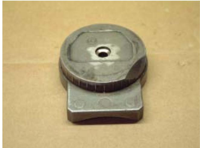
**Fig. 18** Here you can see the notch sanded into the edge of the Gate that is close to the 0.8 OD gear. This relief is excessive for demonstration. You only need about 1/8 of an inch to assure clearance with the gear.
