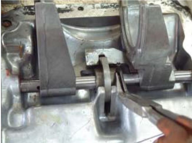
*Fig. 8* Keeping things aligned as you drive this pin back into place is one of the trickier techniques during assembly. Note the vent hole in the front of the shaft. This keeps the oil from being trapped in the Top Plate front Shift Rod bushing.
