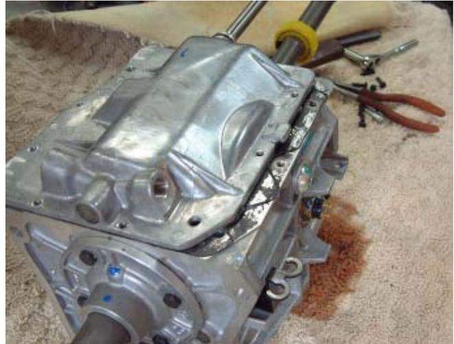
**Fig. 6** The Top Plate slides right to free itself from the internal shift linkage.
