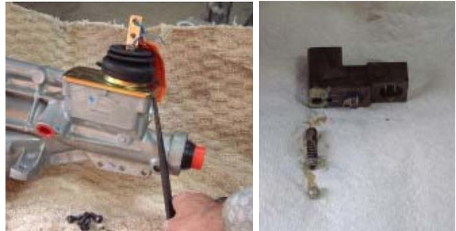
**Fig. 2 & 2A** Tap the shifter loose using a drift. **Fig 2A** shows the Ford shift block and it's components except the roll pin which will stay in side until you drive it out for reuse in the new assembly.
