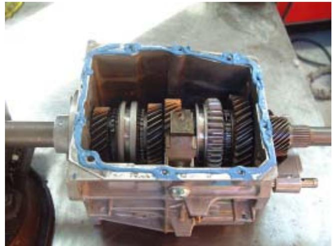
**Fig. 22** Run the bead of RTV around the perimeter and circle the bolt holes.
