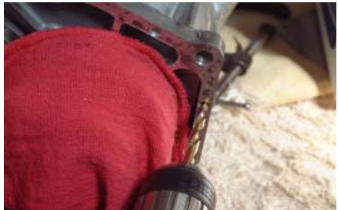
*Fig. 10* Carefully re-drill the tap holes in the case to 1/4" Dia.
