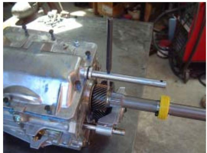
**Fig. 23** You can use a 3/16 drift to shift through the gears and double check that everything is in it's correct place. Make sure you hold the output shaft rear bearing in the case while you check the functions so that the transmission internals don't come out of position.
