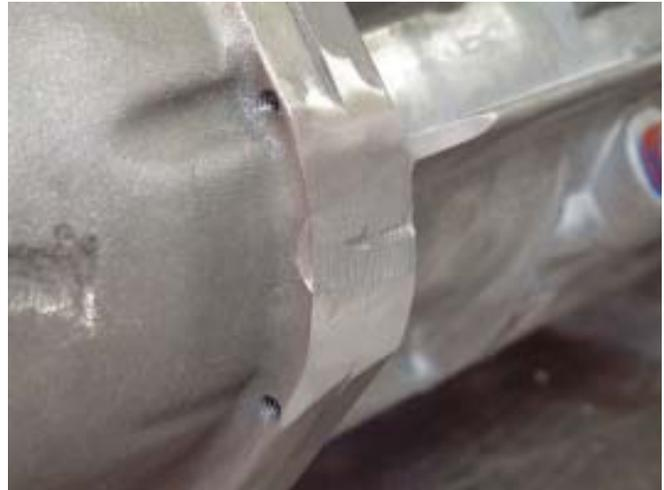
**Fig. 14** Here's the grinding completed before breaking the edges.
