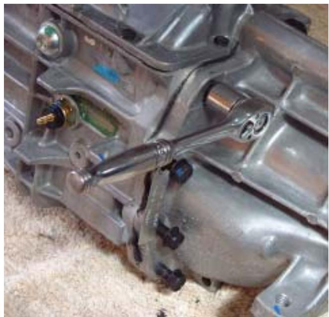
**Fig. 3** Removing the Case Bolts with a 15 mm socket.
