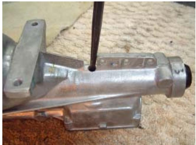
**Fig. 15** Here's one way of getting to the Shift Plate. Locate the approximate center, drill down through both walls and drive the Shift Plate out. The Shift Plate is VERY hard and you won't damage it with a drill bit. Alternatively, depending on tool availability, you can simply saw down to the bottom of the Plate and knock out the remaining aluminum casting with a hammer for access to the Shift Plate.
