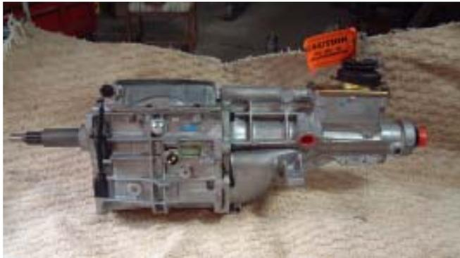
**Fig. 1** This is the Ford Motorsport spec T5 Transmission, p/n M-7003-Z. It is Also known by it's Tremec p/n 1352-249 and has a 2.95 first gear ratio and a 0.668 OD ratio as received.
