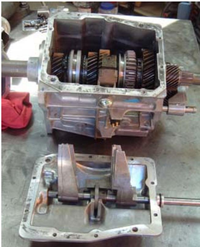
**Fig. 21** This is the level of old RTV removal that I use before re-assembly.
