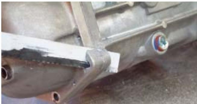
**Fig. 12** Saw through the hole taking most of the ear off.
