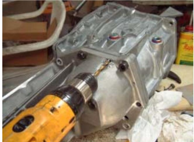
*Fig. 9* Find an appropriate drill and drill motor that will allow you to use the existing #7 holes in the tailhousing to align the drill so that you can drill all the way through the case without "ovalizing" the guide holes.
